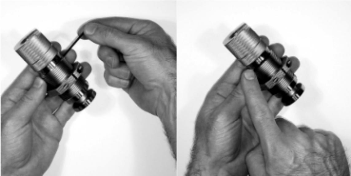
9. While pushing upward so as to fully compress the plunger, tighten down the set-screw on the side, until it just stops, then back off 1/2 turn.
