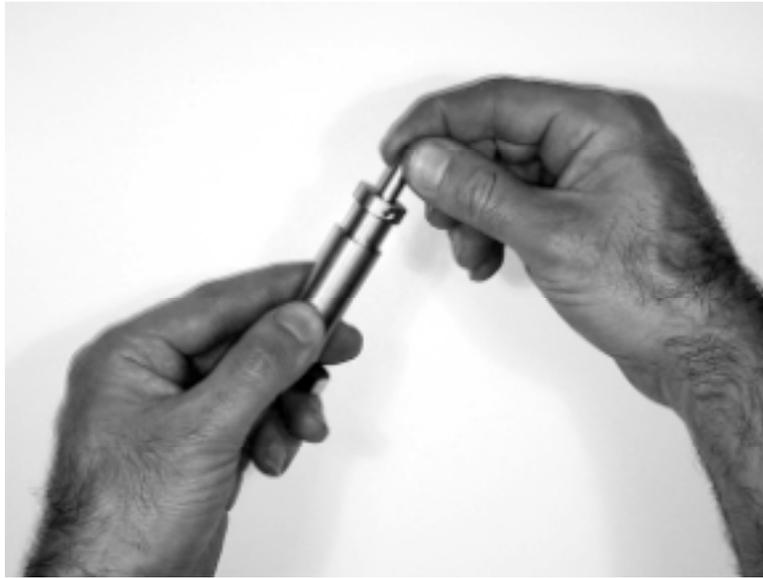
5. Turn the primer pin to lengthen or shorten the overall length. Lengthening will increase the primer seating depth, and shortening it will decrease the seating depth. Turn this pin by hand - don't use a wrench on it.
