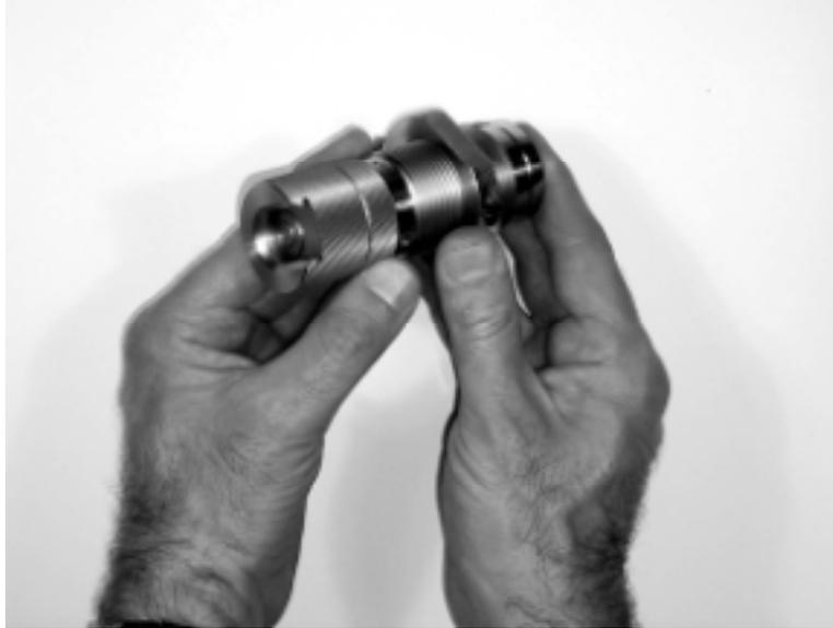
8. Reinstall the spring on the priming pin and put the plunger assembly back in the seater body. Make sure that's in the full up position, the primer pin protrudes out of the center ring. If it doesn't, then you'll have a high primer, which you won't be able to remove from the primer seater.
