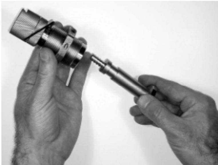
2. Remove the internal plunger assembly and temporarily remove the spring on the priming pin.
