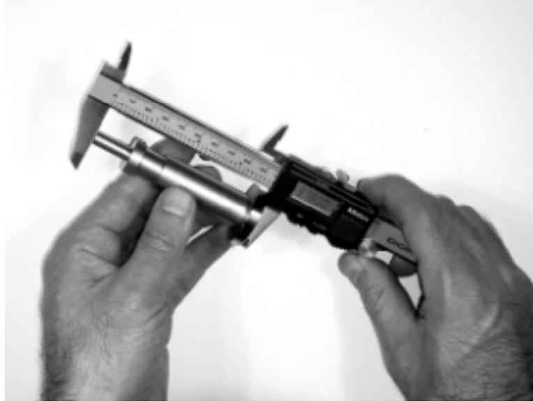
3. Using a caliper, measure and record the overall length of the internal plunger assembly (from the bottom plate to the top of the priming pin). This length was initially set to 3.800"
