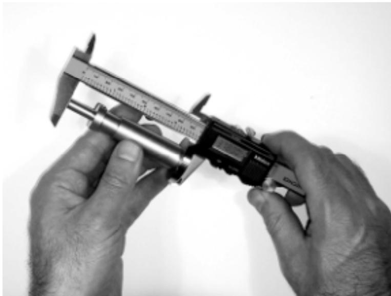
6. Measure the overall length of the plunger assembly with the caliper, and when you're satisfied, tighten down the brass set screw.
